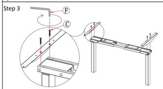
Attach the Side bracket (part 3) to the Crossbeam (part 4) using (part C) Screw M6x45.
