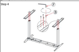
Attach Foot (part 1) to the Lifting leg (part 2) using (part B) Screw M6x16.
