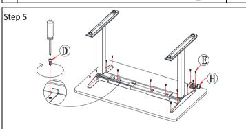
Adjust Crossbeams to the proper position to fit the desktop. Tighten the (part D) Wood screw ST4.8x19 to lock. Attach the Handset (part H) to the underside of the desktop using (part E) Wood screw ST4.2x16.
