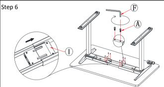
Tighten Crossbeams (part 4) using (part A) Screw M6x10. Attach the Control box (part I) to the Crossbeams.
