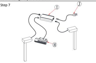
Connect the Lifting legs (part 2), Handset (part H), and the Power cable (part J) to the Control box (part I).
